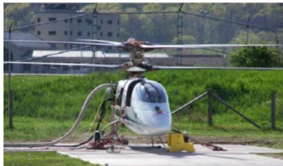
图9 X2地面系留全机响应与稳定性试验 [4] Fig. 9 Ground-tethered test for full-aircraft response and stability of the X2 [4]
